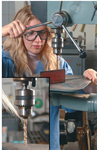
Figure 1-7 Hair does catch on moving machinery. Keep it out of harm's way.
