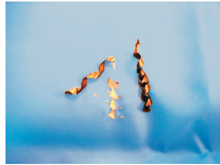
Figure 1-5 Two hot chips melted onto this nylon windbreaker while the center one went completely through to possibly burn the person within!
